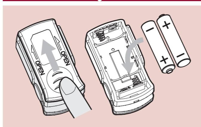
1. Use thumb to slide battery cover out
